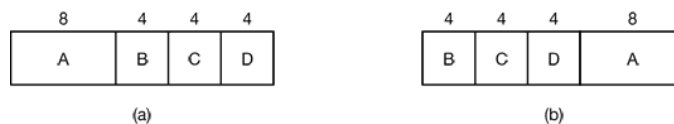
Figure 2-39. An example of shortest job first scheduling. (a) Running four jobs in the original order. (b) Running them in shortest job first order.
