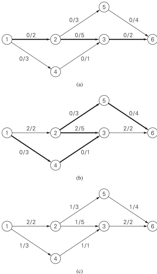
**FIGURE 10.5** Illustration of the augmenting-path method. Flow-augmenting paths are shown in bold. The flow amounts and edge capacities are indicated by the numbers before and after the slash, respectively.
