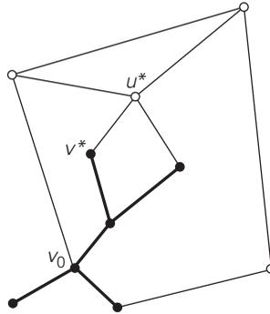
**FIGURE 9.10** Idea of Dijkstra’s algorithm. The subtree of the shortest paths already found is shown in bold. The next nearest to the source  $v_0$  vertex,  $u^*$ , is selected by comparing the lengths of the subtree’s paths increased by the distances to vertices adjacent to the subtree’s vertices.
