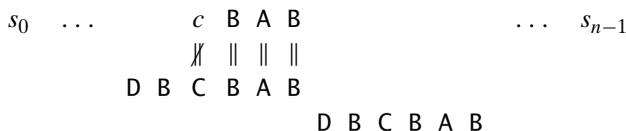
Unfortunately, shifting the pattern by its entire length when there is no other occurrence of  $\text{suffix}(k)$  not preceded by the same character as in its rightmost occurrence is not always correct. For example, for the pattern ABCBAB and  $k = 3$ , shifting by 6 could miss a matching substring that starts with the text's AB aligned with the last two characters of the pattern:
