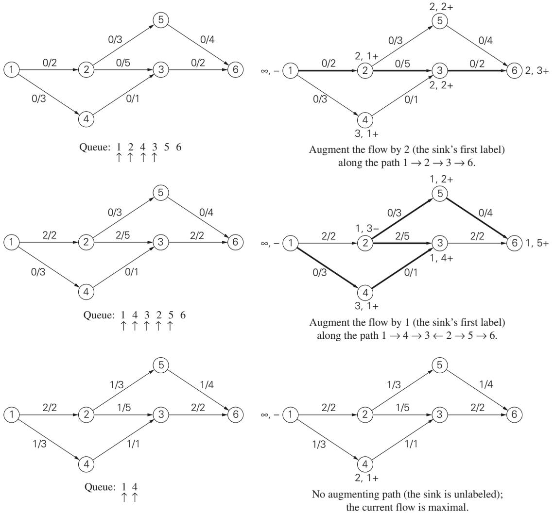
**FIGURE 10.7** Illustration of the shortest-augmenting-path algorithm. The diagrams on the left show the current flow before the next iteration begins; the diagrams on the right show the results of the vertex labeling on that iteration, the augmenting path found (in bold), and the flow before its augmentation. Vertices deleted from the queue are indicated by the ↑ symbol.
