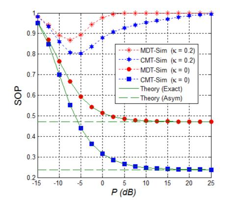
Figure 6.2. End-to-end secrecy outage probability (SOP) as a function of P in dB when  $P \in [-15 \text{ dB}, 25 \text{ dB}]$ ,  $\mu = 0.5, M = 4, R_s = 1, \kappa \in \{0, 0.2\}, (x_{PU}, y_{PU}) = (-0.5, -1) \text{ and } (x_E, y_E) = (0.5, 0.5).$
