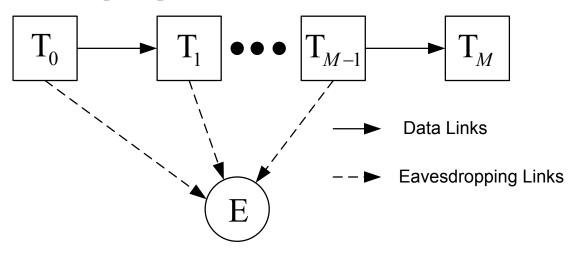
Figure 4.3. System model of Multi-hop Cooperative Transmission Protocol.
