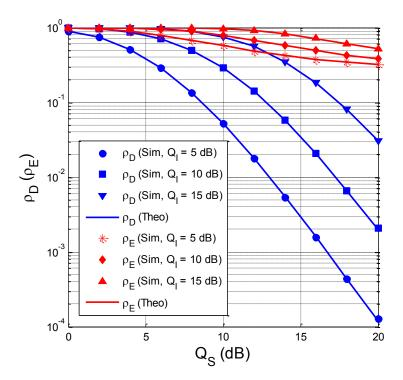
Figure 8.2.  $\rho_{\rm D}$  and  $\rho_{\rm E}$  as a function of  $Q_{\rm S}$  in dB when M = 3,  $\alpha = 0.3$ ,  $\kappa_{\rm D}^2 = \kappa_{\rm E}^2 = 0.1$  and  $C_{\rm th} = 0.75$ .
