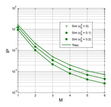
Figure 8.6. IP as a function of M when  $Q_{\rm S} = Q_{\rm I} = 20 \, dB$ ,  $\kappa_{\rm D}^2 = 0.2$ ,  $\alpha = 0.3$ ,  $N_{\rm th} = 20 \, and \, C_{\rm th} = 0.5$ .
