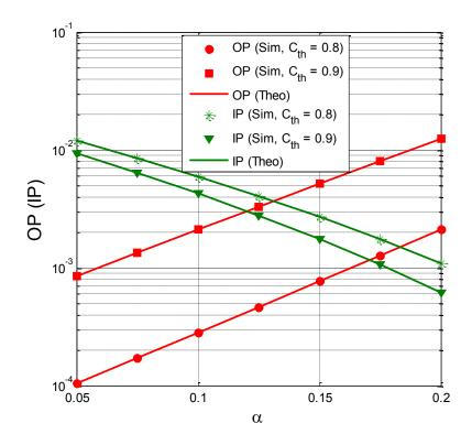
Figure 8.8. OP and IP as a function of  $\alpha$  when  $Q_{\rm S} = Q_{\rm I} = 15 \, dB$ , M = 4,  $\kappa_{\rm D}^2 = \kappa_{\rm E}^2 = 0$  and  $N_{\rm th} = 16$ .
