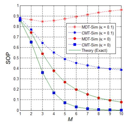
Figure 6.3. End-to-end secrecy outage probability (SOP) as a function of M when P = 5 dB,  $\mu = 1$ ,  $M \in [1,10]$ ,  $R_S = 0.5$ ,  $\kappa \in \{0,0.1\}$ ,  $(x_{PU}, y_{PU}) = (-0.5, -0.5)$  and  $(x_E, y_E) = (0.5, 0.5)$ .
