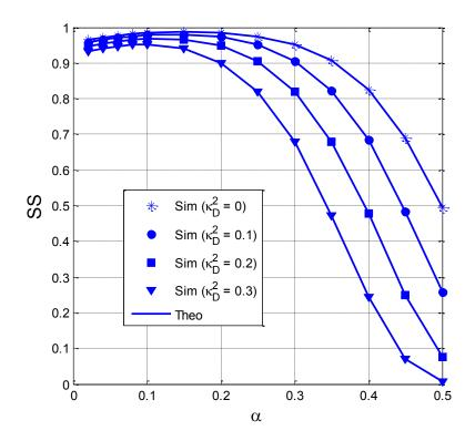
Figure 8.5. SS as a function of  $\alpha$  when  $Q_{\rm S} = Q_{\rm I} = 15 \, dB$ , M = 3,  $\kappa_{\rm E}^2 = 0.1$ ,  $N_{\rm th} = 15 \, and \, C_{\rm th} = 0.7$ .
