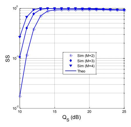
Figure 8.4. SS as a function of  $Q_{\rm S}$  in dB when  $Q_{\rm I} = 10 \, dB$ ,  $\alpha = 0.1$ ,  $\kappa_{\rm D}^2 = 0.1$ ,  $\kappa_{\rm D}^2 = 0$ ,  $N_{\rm th} = 20$  and  $C_{\rm th} = 1.5$ .
