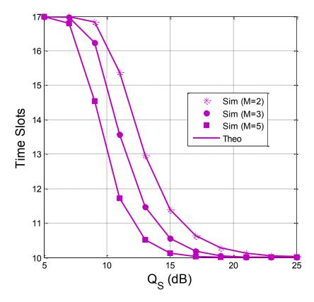
**Figure 8.9.** Average number of time slots as a function of  $Q_{\rm S}$  in dB when  $Q_{\rm I} = 10 \, dB$ ,  $\alpha = 0.2$ ,  $\kappa_{\rm D}^2 = \kappa_{\rm E}^2 = 0.05 \, N_{\rm th} = 17 \, and \, C_{\rm th} = 1.$
