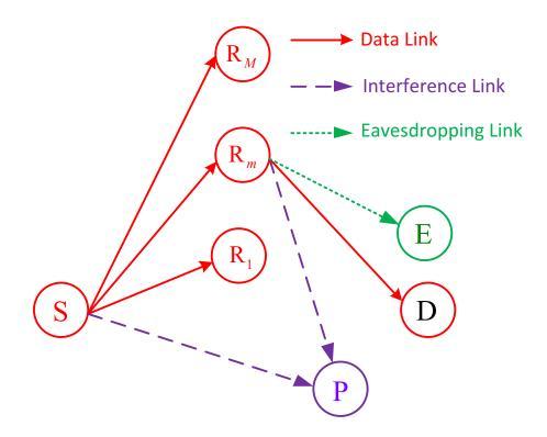
Figure 5.1. Secure communication in dual-hop underlay cognitive radio networks.
