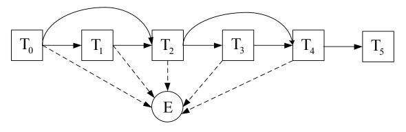
Figure 4.5. Cooperative transmission in the MCT protocol when M=5.
