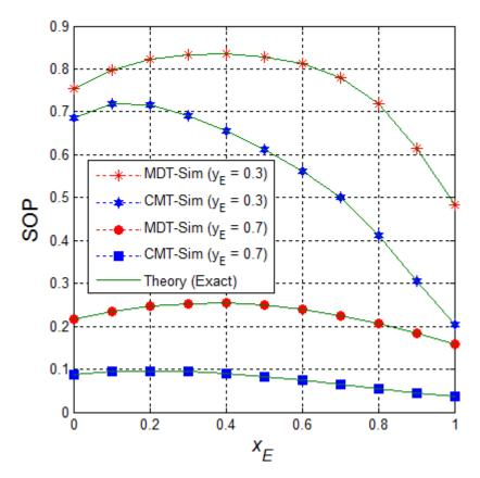
Figure 6.5. End-to-end secrecy outage probability (SOP) as a function of  $x_E$  when P = 10 dB,  $\mu = 1$ ,  $M = 4, R_S = 1, \kappa = 0, (x_{PU}, y_{PU}) = (-0.5, -1), x_E \in [0,1] \text{ and } y_E \in \{0.3, 0.7\}.$
