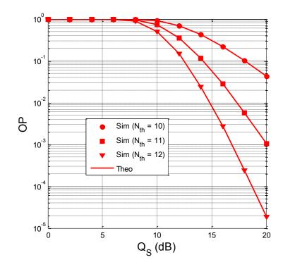
**Figure 8.3.** OP as a function of  $Q_{\rm s}$  in dB when  $Q_{\rm l} = 7.5 \, dB$ , M = 2,  $\alpha = 0.1$ ,  $\kappa_{\rm D}^2 = \kappa_{\rm E}^2 = 0$  and  $C_{\rm th} = 1$ .
