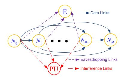
Figure 6.1. System model of the cooperative multi-hop transmission protocol in an underlay CR network.
