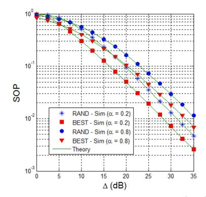
**Figure 7.3.** Secrecy outage probability (SOP) as a function of the transmit SNR  $\Delta(P/N_0)$  in dB when M = 3,  $K_1 = 2$ ,  $K_2 = 3$ ,  $K_3 = 2$  and  $\kappa^2 = 0$ .
