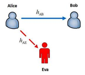
Figure 4.1. A fundamental system model of physical-layer security (PLS).
