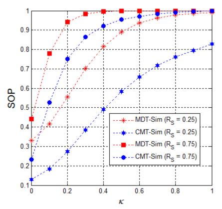
Figure 6.4. End-to-end secrecy outage probability (SOP) as a function of  $\kappa$  when P = 0 dB,  $\mu = 1, M = 4, R_s \in \{0.25, 0.75\}, \kappa \in [0,1], (x_{PU}, y_{PU}) = (-0.5, -1) and (x_E, y_E) = (0.5, 0.5).$
