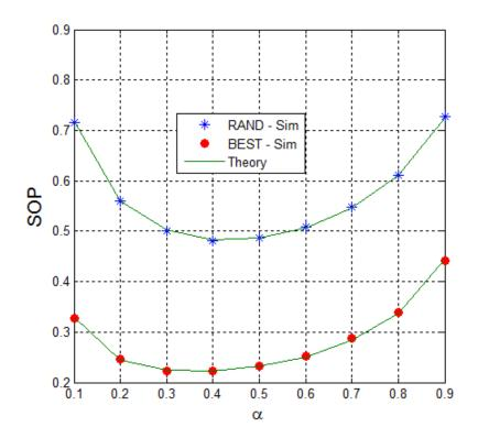
Figure 7.5. Secrecy outage probability (SOP) as a function of the fraction  $\alpha$  when  $\Delta = 10 \, dB$ , M = 4,  $K_n = 4 \, \forall n \text{ and } \kappa^2 = 0$ .
