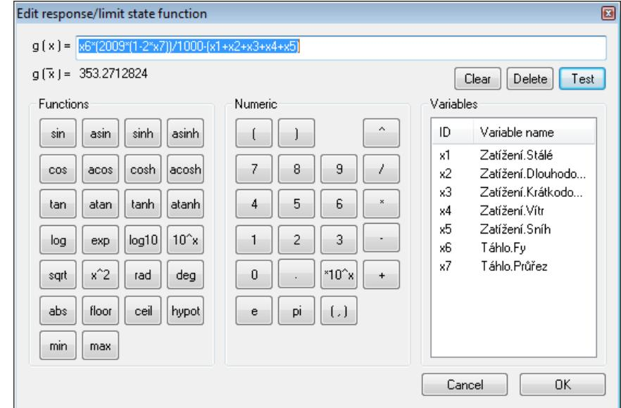
**Freet:** Definition of the computing model and substituting the generated permutations in this model.
