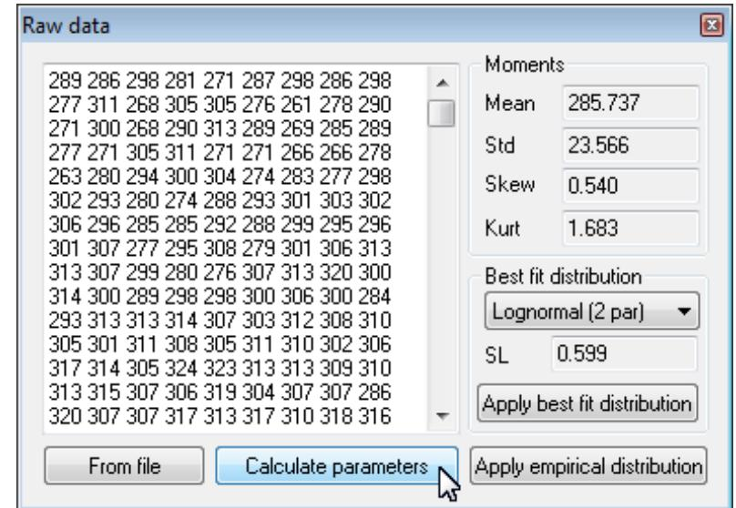
Selecting the appropriate parametric distribution for the specified measurements.
